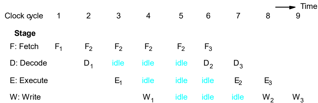
(b) Function performed by each processor stage in successive clock cycles
